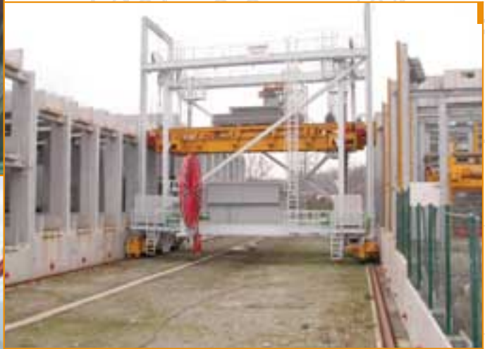
2 Storage and retrieval machine in concrete manufacturing – This custom-built design moves stacks of concrete up to 50,000 kg in weight with four synchronised R. STAHL hoists.
