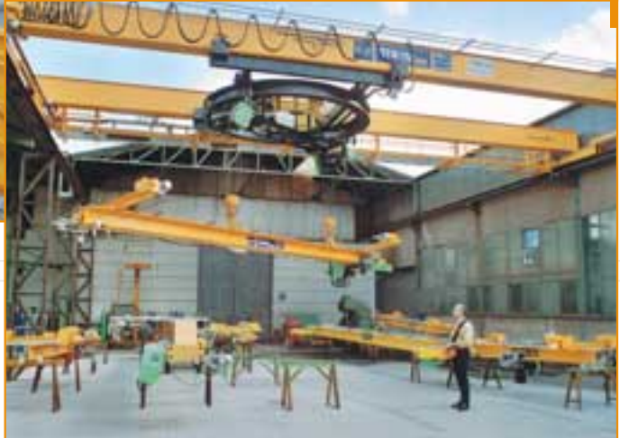
3 Ship outfitting – This double girder overhead travelling crane with 40,000 kg S.W.L. can be used even in rough seas thanks to its special equipment geared to marine use.
