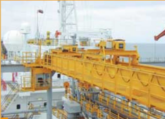
3 Ship outfitting – This double girder overhead travelling crane with 40,000 kg S.W.L. can be used even in rough seas thanks to its special equipment geared to marine use.
