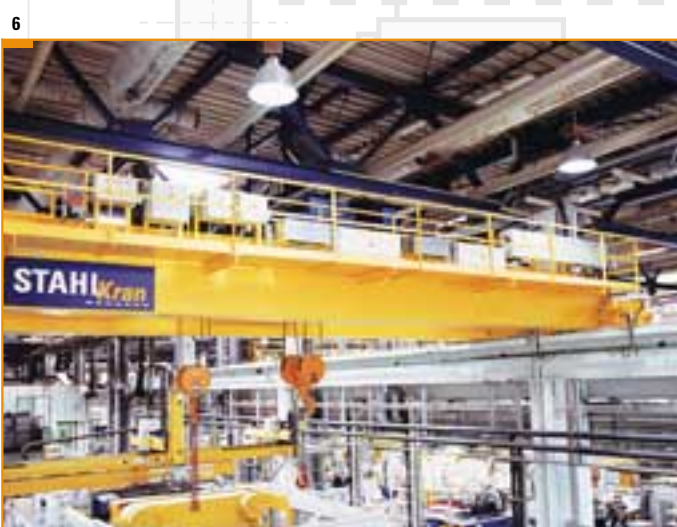
6 Motor industry – Here double girder overhead travelling cranes with extensive equipment for safe working with heavy loads are in use. Lighter loads are moved quickly with a fast hoist, heavy and bulky loads are lifted by a slow-moving wire rope hoist. The stepless control of the drives and the maintenance platform along the crane bridge are particularly convenient.
