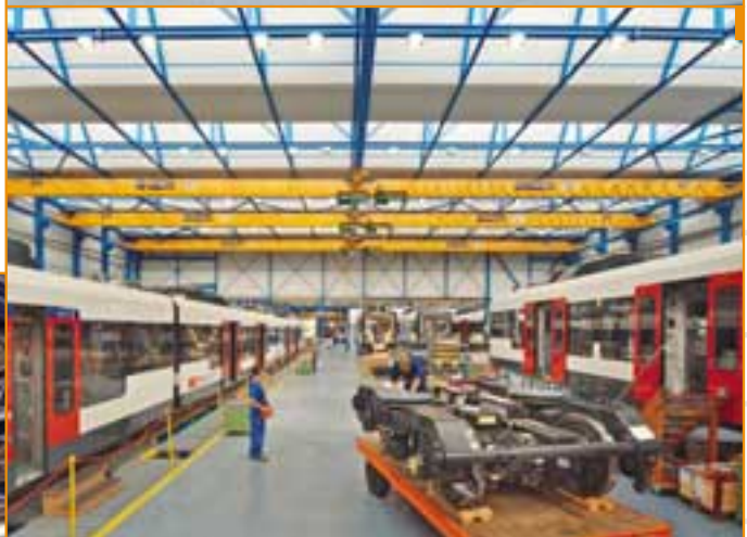
6 Motor industry – Here double girder overhead travelling cranes with extensive equipment for safe working with heavy loads are in use. Lighter loads are moved quickly with a fast hoist, heavy and bulky loads are lifted by a slow-moving wire rope hoist. The stepless control of the drives and the maintenance platform along the crane bridge are particularly convenient.
